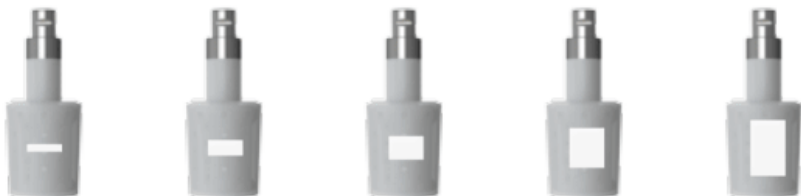
PTFE/PFA lined plug: linear control characteristics
